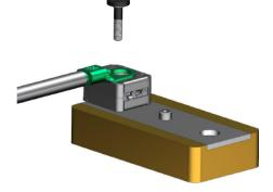
All tests were performed mounting the Zcase on the left or right side of the metal bar, as shown in the picture. A 50mm<sup>2</sup> wire was used as current feed for all the ratings, while the output wire size was according to the table on
